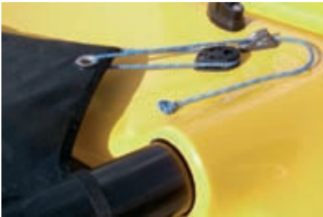
Tightening the trampoline: nothing simpler with the system developed by the New Zealand-based builder.
