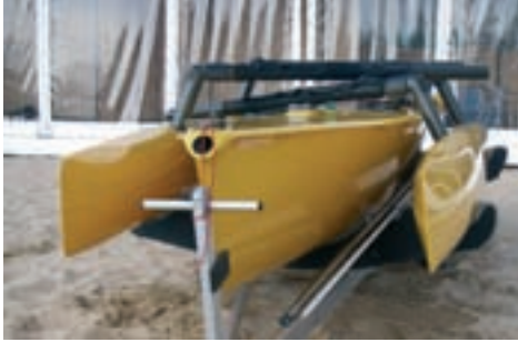
On its launching trolley, the Weta is only 1.5m wide.
